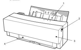
Front cover release button - Pressing this button opens the front cover. The front cover will need to be opened when there is a paper jam or when
